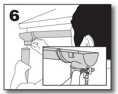
Slide downpipe onto stop-end outlet. For flexible downpipes, the pipe needs to go to the very top, widest part of the outlet and tightened by the clamp key, see inset diagram.
