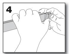
When all brackets are in place, clip the stop-end to the gutter. Some force is necessary in order to compress the rubber seal. A smear of washing up liquid or silicone grease/spray on the seal may help if required.
